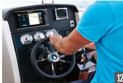
Helm with hydraulic steering, SmartCraft, dual 9" GPS/Chart plotter, stereo and 12v outlet
